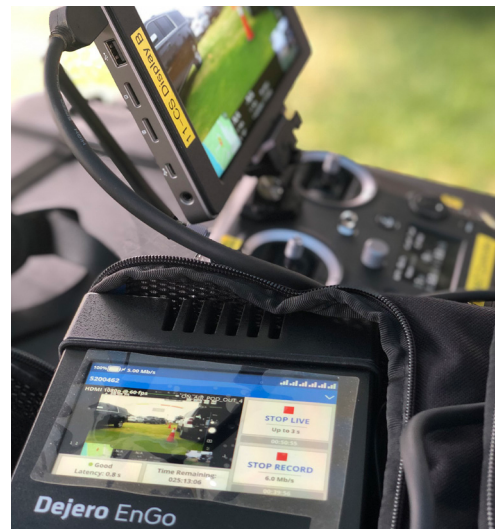
Dejero EnGo 260 mobile transmitter fed real-time video from a drone back to the San Diego Police Department command post and HQ over cellular for situational awareness at the US Open in Torrey Pines.
